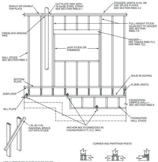
APPLY APPROVED SHEATHING OR BRACE EXTERIOR WALLS WITH 1 IN. BY 4 IN. BRACES LET INTO STUDS AND PLATES AND EXTENDING FROM BOTTOM PLATE TO TOP PLATE, OR OTHER APPROVED METAL STRAP DEVICES INSTALLED IN ACCORDANCE WITH THE MANUFACTURER'S SPECIFICATIONS. SEE SECTION R602.10.
